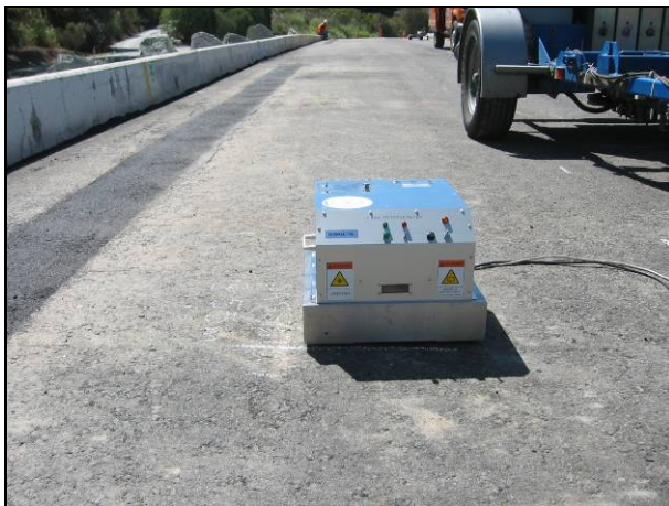
Figure 2.52: Caltrans Portable Skid Tester.
