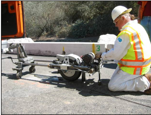
Figure 2.52: Caltrans Portable Skid Tester.
