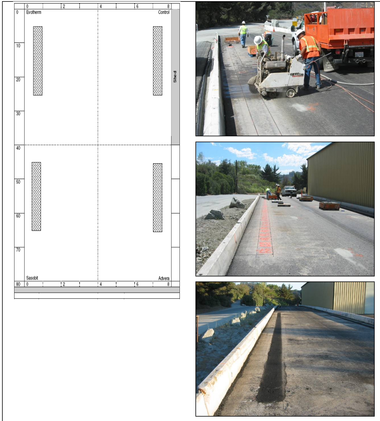
Figure 2.56: Test track sampling plan and sample removal.
